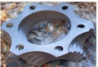
harde ned steel checking iig made by PTL
