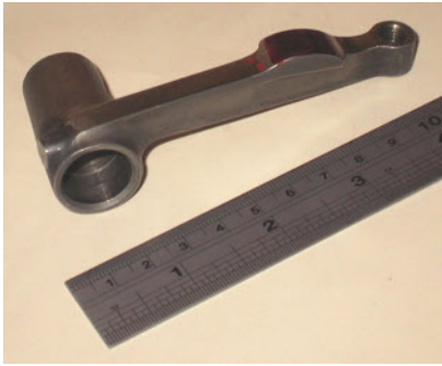
1 of 96 rocker arms repaired by PTL to restore old aircraft engines
