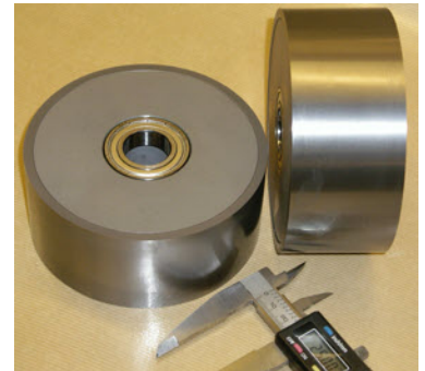
rollers with tungsten carbide outer rings fitted against wear
